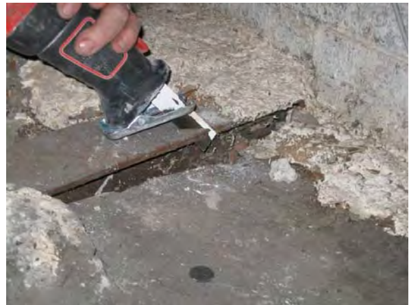
Figure C225. Removal of sample S1 from top flange of 9" deep wrought iron attic floor framing beam.
