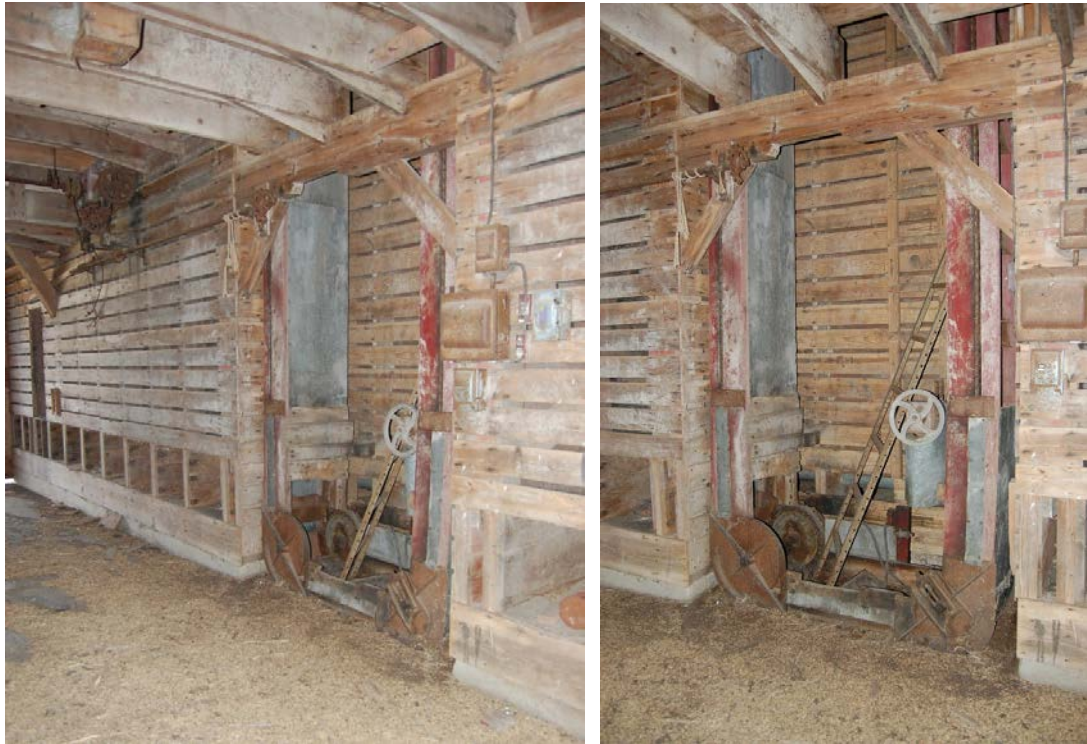
Figure 136. Two views of the elevator mechanism. This elevator system was not original to the corn crib, and although it may have been originally installed to handle ear corn, it probably was added to the structure at the same time that it was converted to shelled corn.
