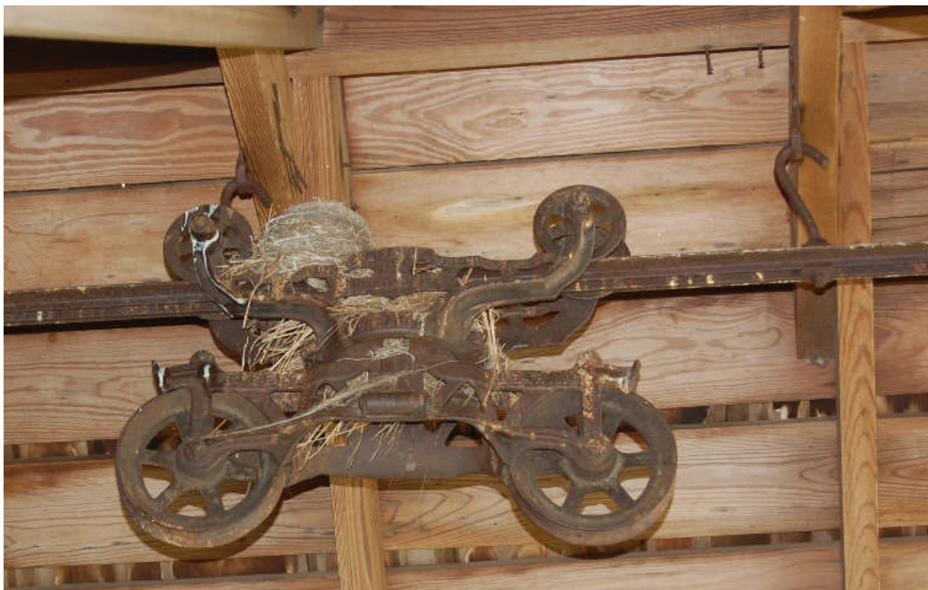
Figure 114. The extremely large, two-story hayloft was made practical with the aid of a mechanical hay carrier (and/or unloader). This metal-track hay carrier was marked "The F. E. MYERS & BRO. CO. / O.K. / UNLOADER / ASHLAND, O. / STEEL BEARING." It also had the numbers H 427 embossed on a pulley wheel, and another partially illegible number ("?92") embossed on the main mechanism.
