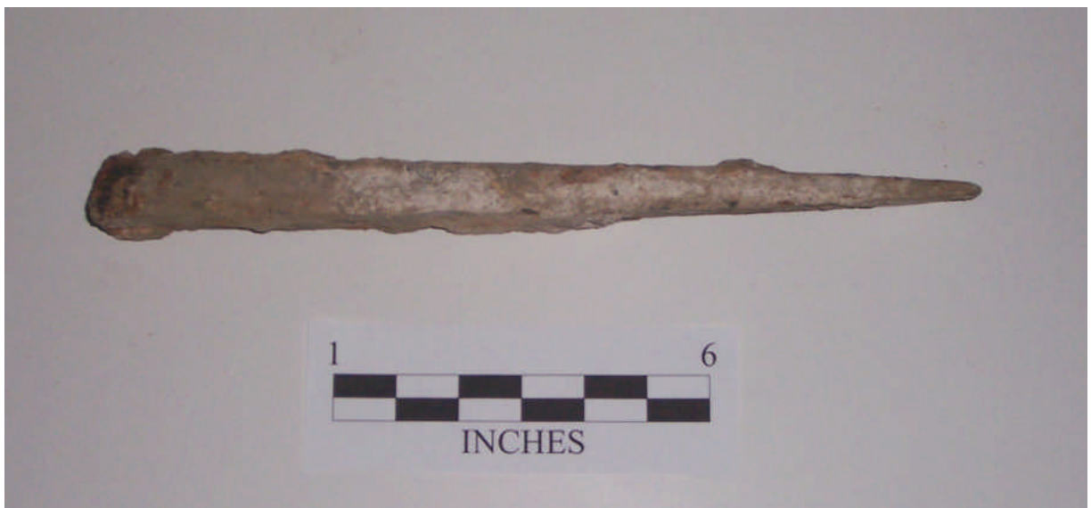
Views of a wedge-like piece of hardware found between the stone courses near the base of the dam at its eastern end, showing it as found in situ and laid flat (TOP) and from the side after removal (BOTTOM). This cast iron piece measures 1-1/2" wide and 14" long. The reason for it being left between the stone coursing is not clear, though one possibility is that it was inserted initially to serve as a type of hanger or bracket (possibly during the course of the dam's construction) and later was driven in flush with the stonework to prevent people or objects from hanging up on it.
