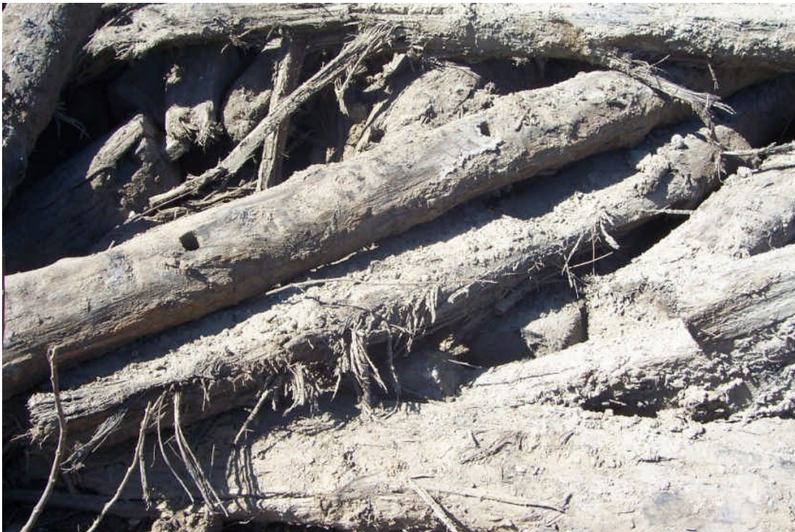
Photographs of the large timbers removed from below the stone abutment on the west end of the River Street Bridge. The timbers were hand hewn to varying degrees and showed evidence of having been fitted together by a number of methods, including notching, mortise and tenon, and wood dowels. They may represent the remains of an earlier timber bridge abutment or timbers salvaged from another structure, which were later reused as footing material for the stone abutment associated with the circa 1890-1900 bridge.
