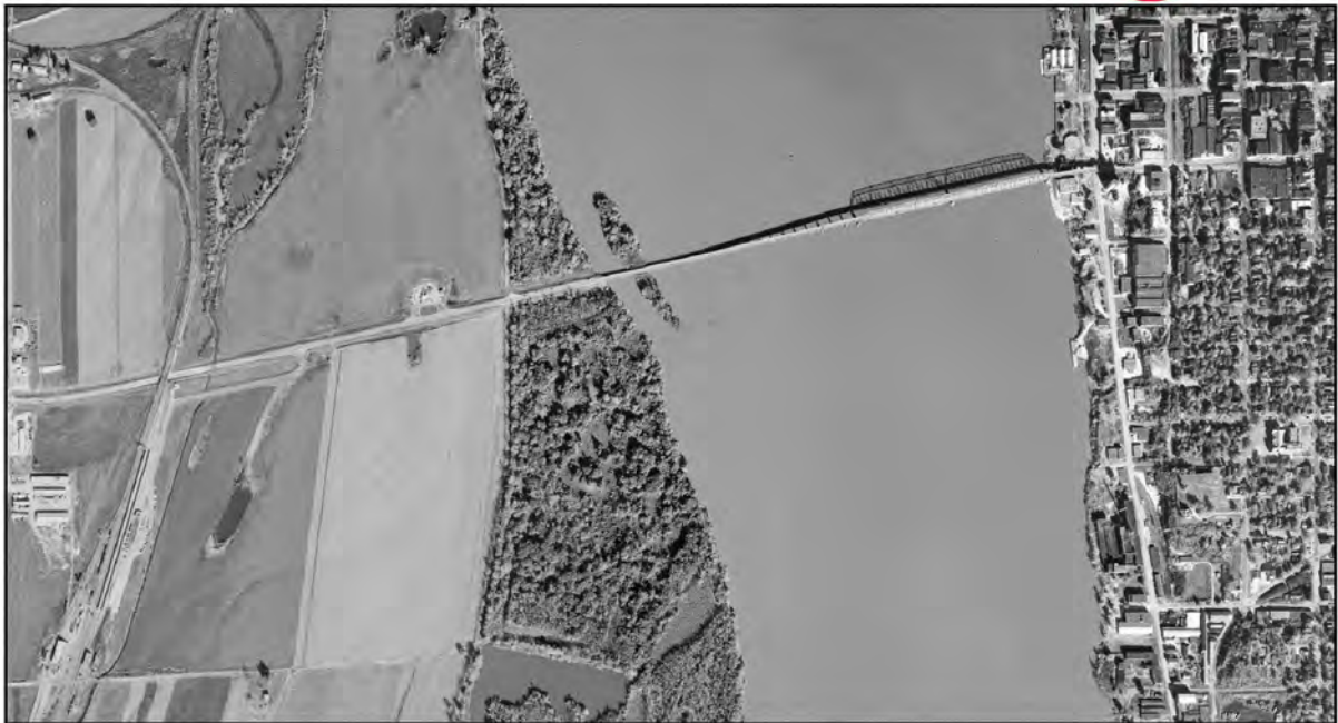
Figure 22: These pictures, taken nineteen years apart illustrate the bridge and its evolving setting. Note that the 1957 image is highlighted by the shadow that illustrates the structure's continuous top chord (Illinois Historic Aerial Photography, Image SA-16-1498, 15 July 1938 and Image SA-2T-115, 27 October 1957, Viewed on 09 December 2025 at http://maps.isgs.illinois.edu/ilhap ).
