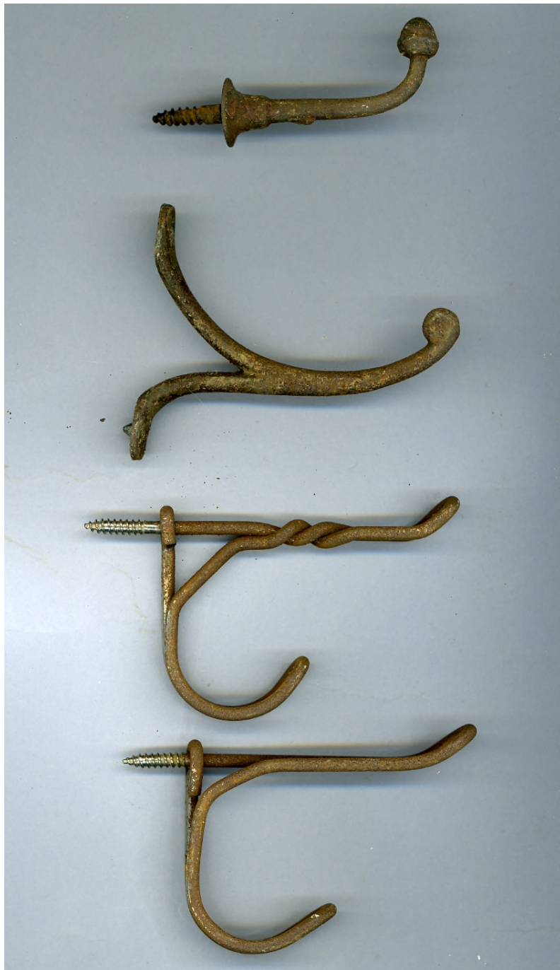
Figure 14. Clothes hooks from the Moore House, St. Clair County, Illinois. Early clothes hooks were cast iron, as represented by the upper two examples. Note the acorn finial on the upper hook. The later nineteenth and twentieth century hooks were constructed of twisted iron wire with screw threads cut onto one end. The hooks are reproduced at 75% their actual size.
