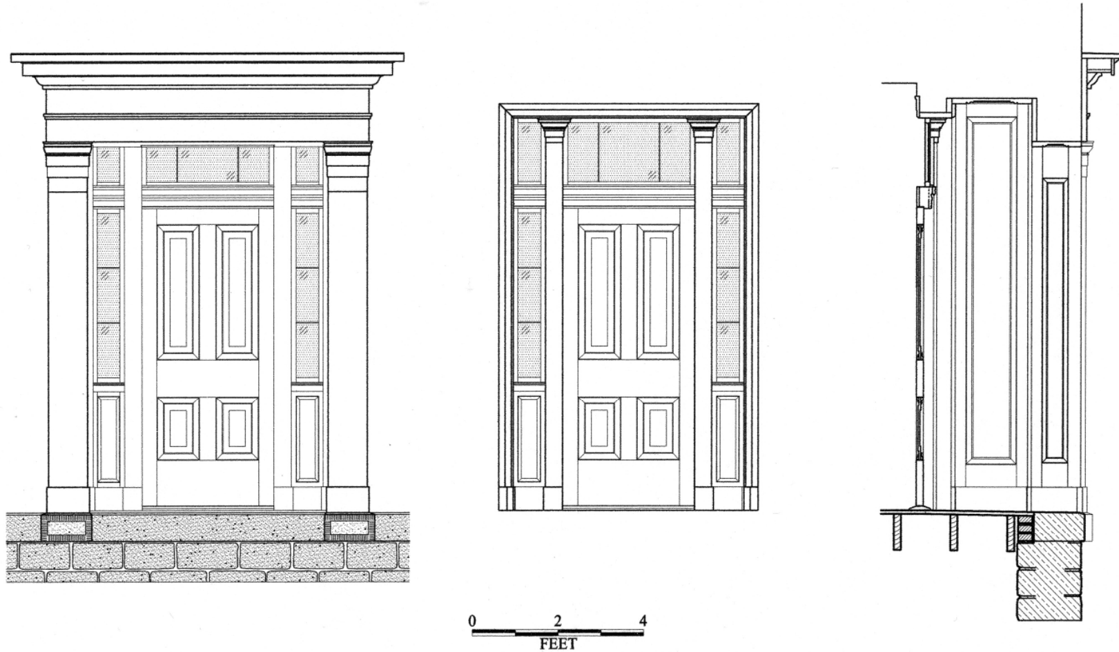
Figure 11. Drawings of the formal entrance on the north elevation of the residence. This entrance is quite ornate and is recessed within the body of the house. The drawing at LEFT shows the front entrance from outside the house, while that in the CENTER illustrates it from within the recessed entranceway. The drawing at RIGHT is a sectional view through the entranceway. Note the paneled side walls.
