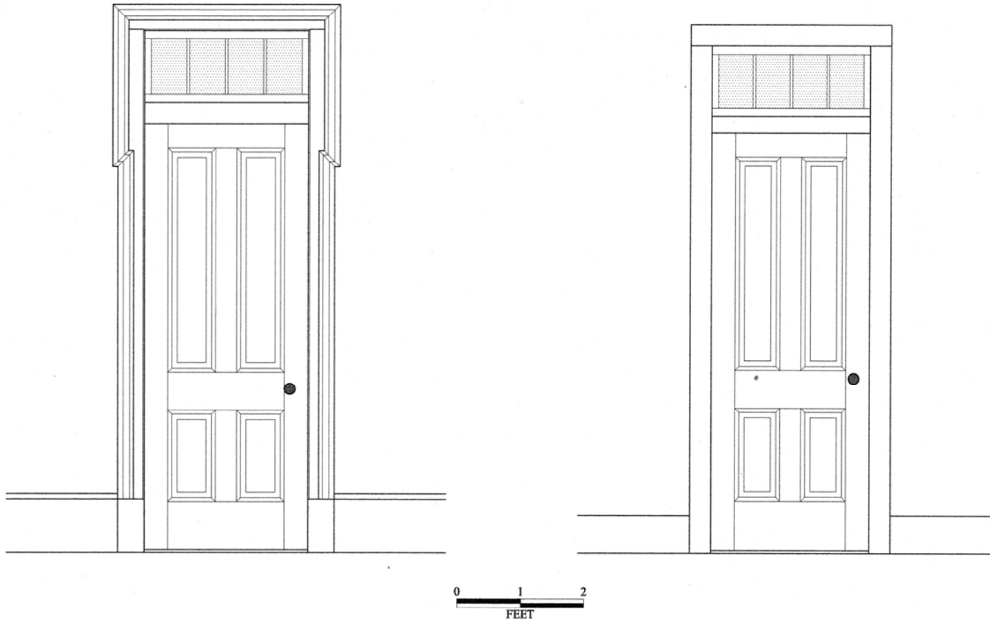
Figure 20. Door details, illustrating the difference in character between the doorways and associated trim in the hotel building. The image at LEFT is representative of the doorways on the first and second floors of the main block, while that at RIGHT is representative of the doorways on the third floor of the main block and second floor of the rear wing. Note the simpler trim used on the latter.
