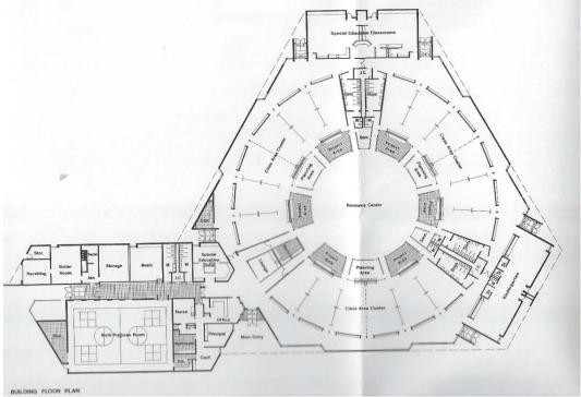
Figure 50: Drawing and floor plan for Parkwood Elementary School in Hanover Park, designed by Schmidtke and Layer Architects, 1969.
