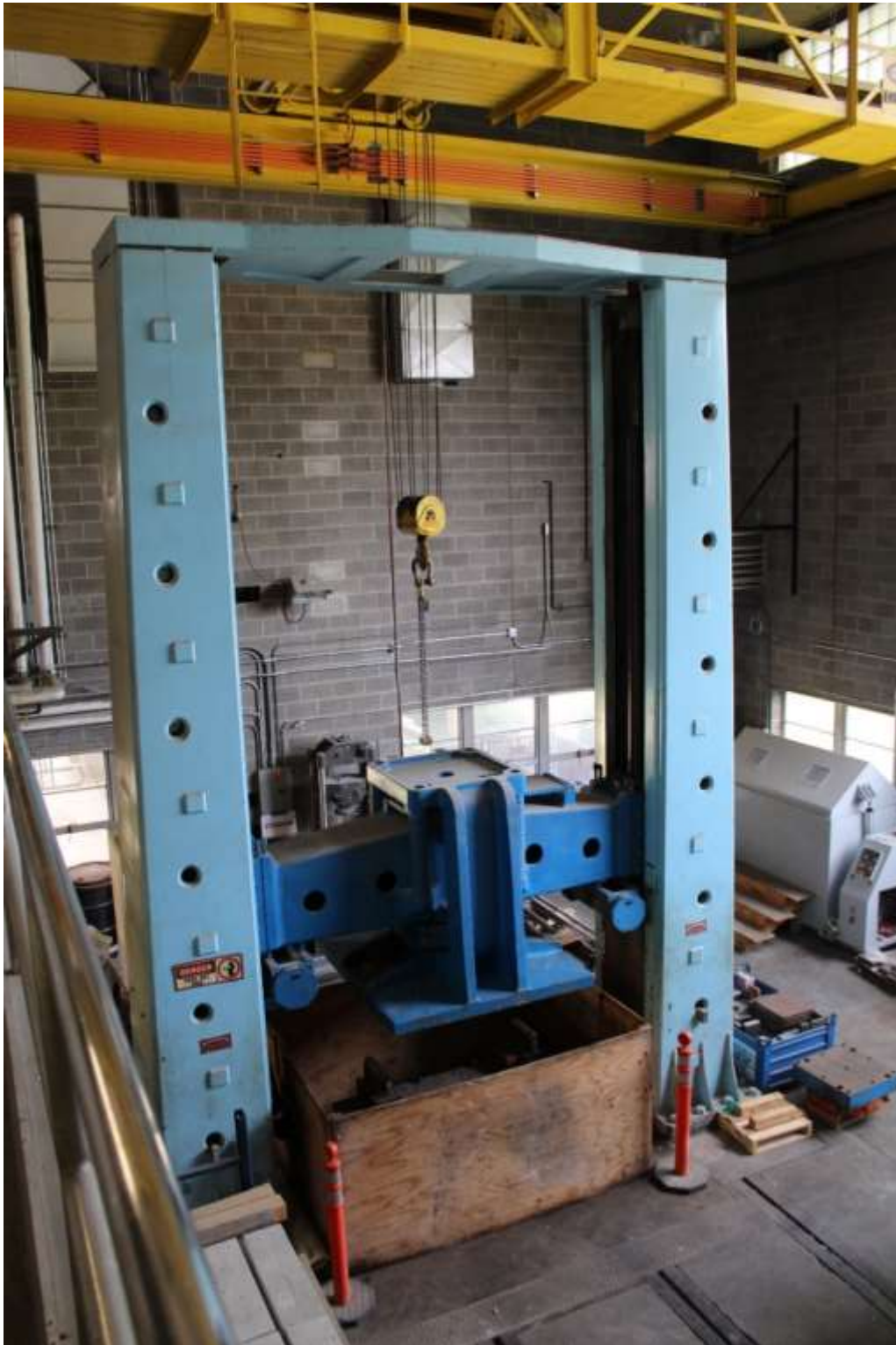
Photograph 41: Million pound testing machine.
