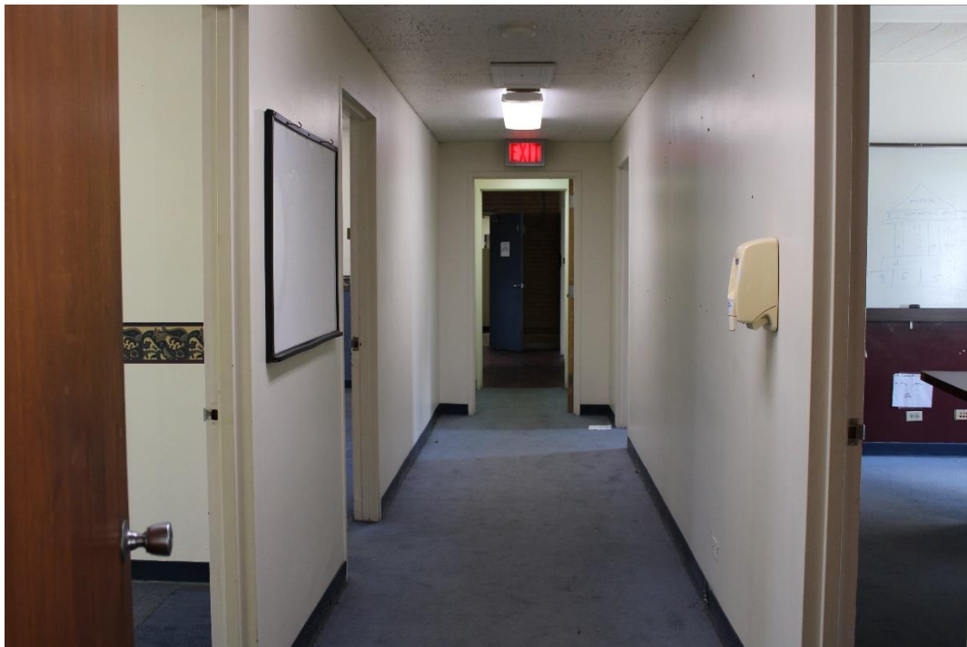
Figure 31: Double-loaded corridor on first floor.
