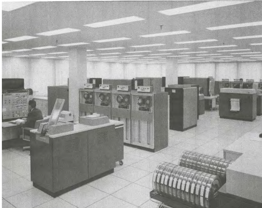
Figure 74: Computer room in North Plaza Complex, 1967. Machines were placed on a metal floor, which was removable in sections to allow access for electrical service. Source: Allstate Corporate Archive.
