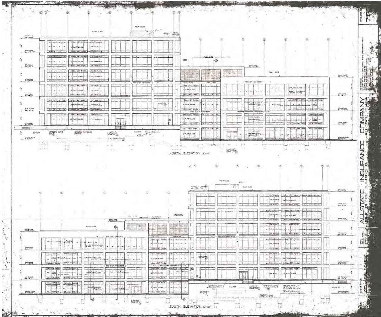
Figure 48: Schmidt, Garden & Erikson, Sheet A8, South Plaza Complex’s G building – North and South Elevations, November 15, 1972.
