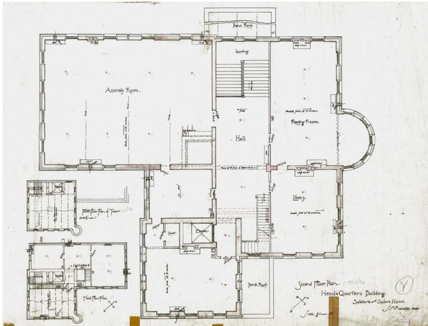
Second Floor Plan, Soldier's And Sailor's Home, Headquarters Building (S. M. Randolph, 1885). This sheet also contains the Third Floor Plan, and Fourth Floor of Tower plan as well.
