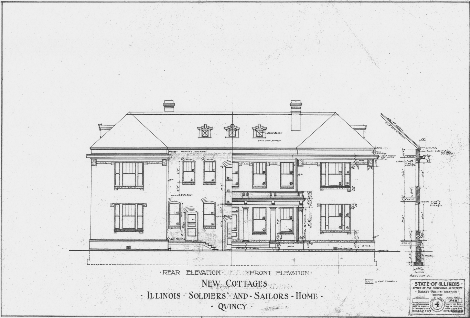
Figure 4. Front and rear elevation views of Building 11/Rowland Barracks, as originally designed (1905). A sectional through the west wall of the south wing also is shown.
