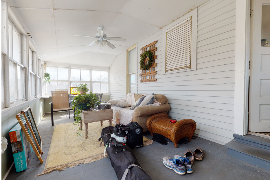
23: General view of second floor sleeping porch, looking east. Wood clapboard siding is right of center, and painted wood flooring and framing remain partially visible throughout.
