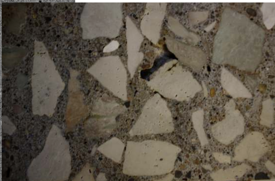
FIG. 21 Core 1 (Nilwood/Girard); lapped surfaced shown on lower half of the core sample.
