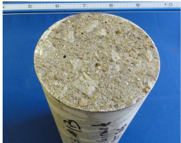
Figure 3. Core 1B; weathered top surface of the core as received.
