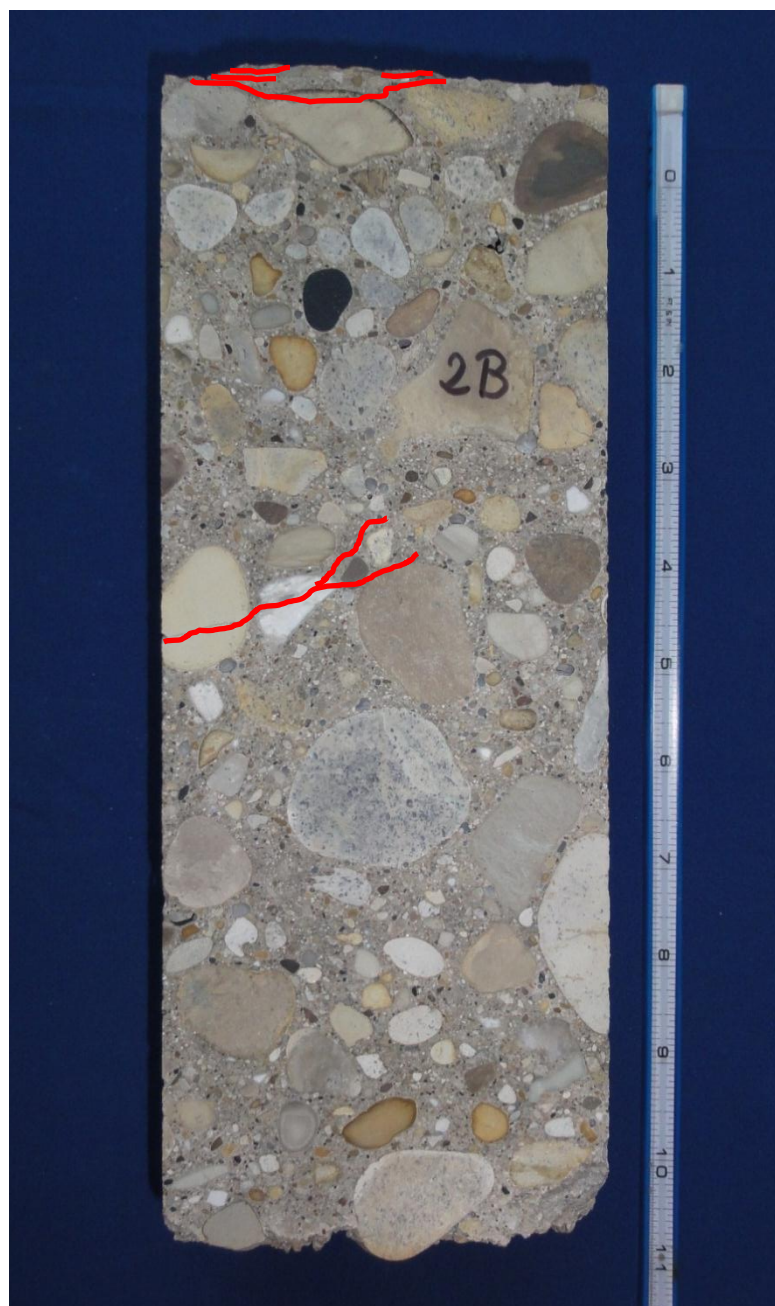
Figure 14. Lapped section of Core 2B. Crack locations are marked in red.
