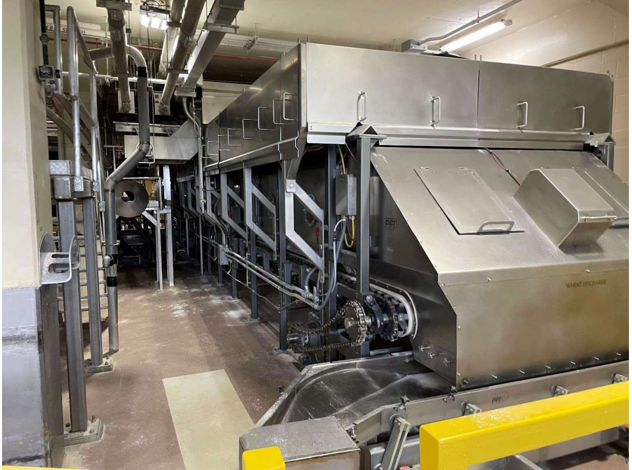
Crisped rice storage conveyor 5 th floor.
