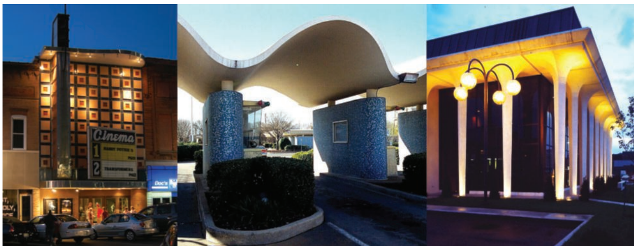
Figure 5: Structural innovations and dramatic space-age-inspired design also appeared on Main Street in a style named Exaggerated Modern by Chester Leibs in his seminal book Main Street to Miracle Mile . On the left the Taylorville, Illinois cinema was completely refaced in the mid-century with polychrome porcelain enamel panels, swooping stainless steel and aluminum canopy and cornice, and dramatic pylon. In the middle, the elegant Oklahoma City Central Motor Bank drive-up, built in 1959, combines a thin-shell concrete roof with bright blue mosaic tile encased piers. On the right, precast concrete columns surround a darkly glazed curtain wall on this Moline, Illinois bank, designed by John Van Scheltema, of the Illinois Bank Building Corporation in the 1970s.
