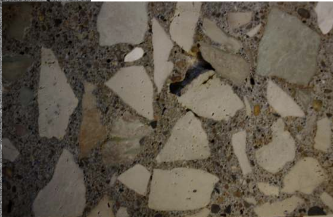
FIG. 21 Core 1 (Nilwood/Girard); lapped surfaced shown on lower half of the core sample.
