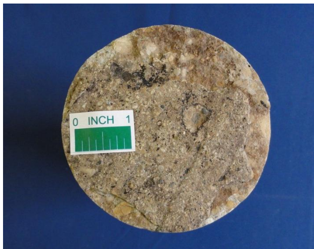
Figure 5. Core 2B; partially weathered, scaled top surface of the core as received.
