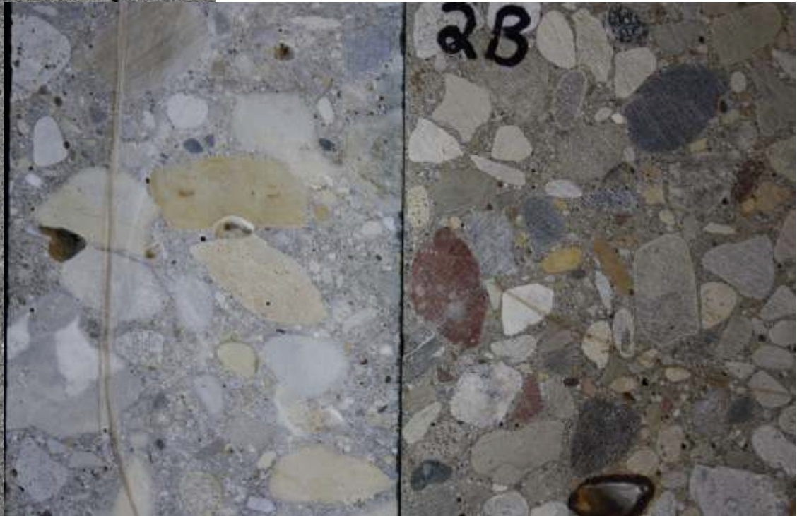
FIG. 27 Currently available crushed limestone (left) compared to aggregates in Core 1 (samples from Ozinga).
