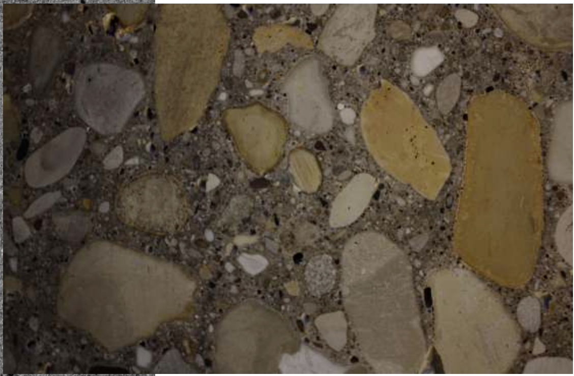
FIG. 23 Core 2 (Pontiac/Dwight); lapped surfaced shown on lower half of the core sample.
