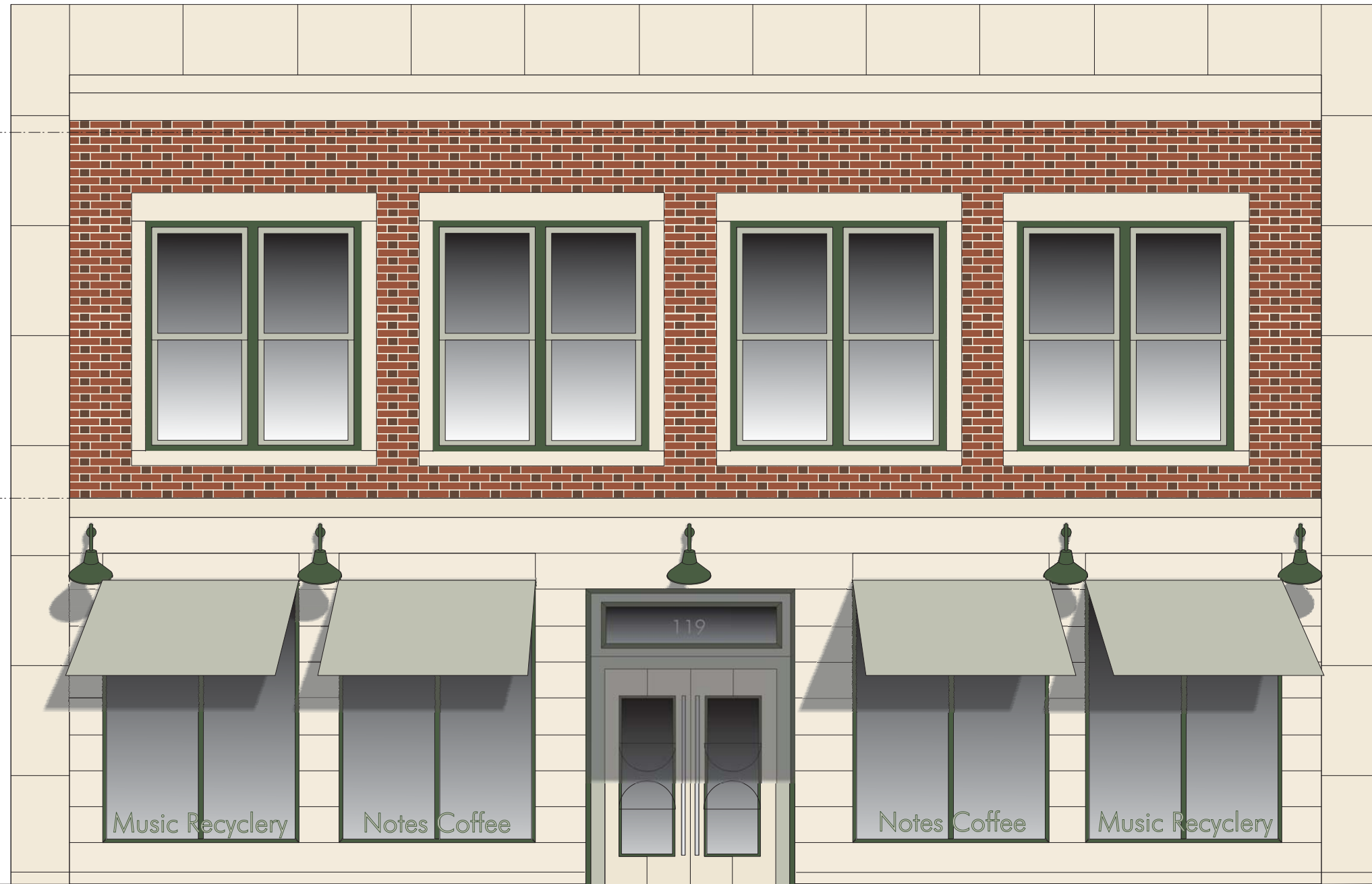
PROPOSED DESIGN WITH DOUBLE-HUNG WINDOWS ON SECOND FLOOR. FIRST-FLOOR DISPLAY WINDOWS EXTEND TO CEILING.
