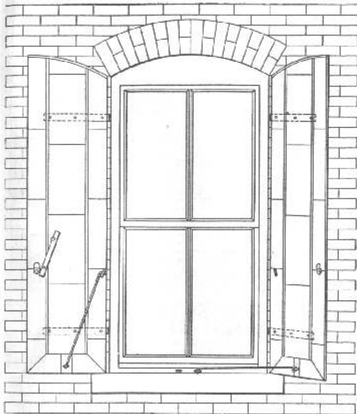
No. 275. TIN CLAD FIRE SHUTTERS.
