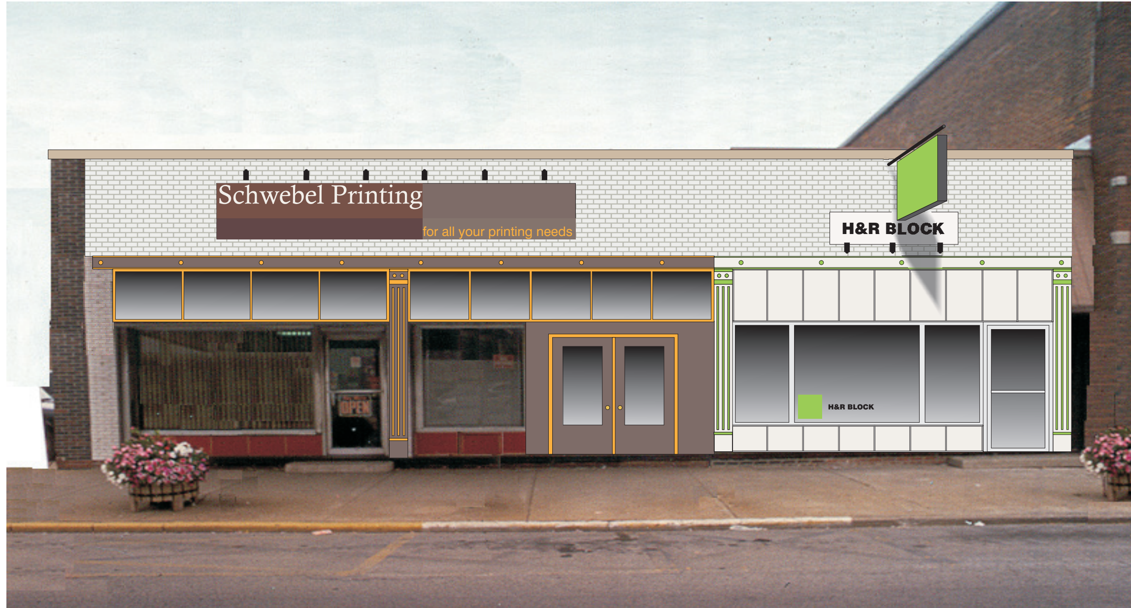
PROPOSED DESIGN. AWNINGS NOT SHOWN. HANGING BLOCK SIGN W/ UP-LIT NAME BOARD
