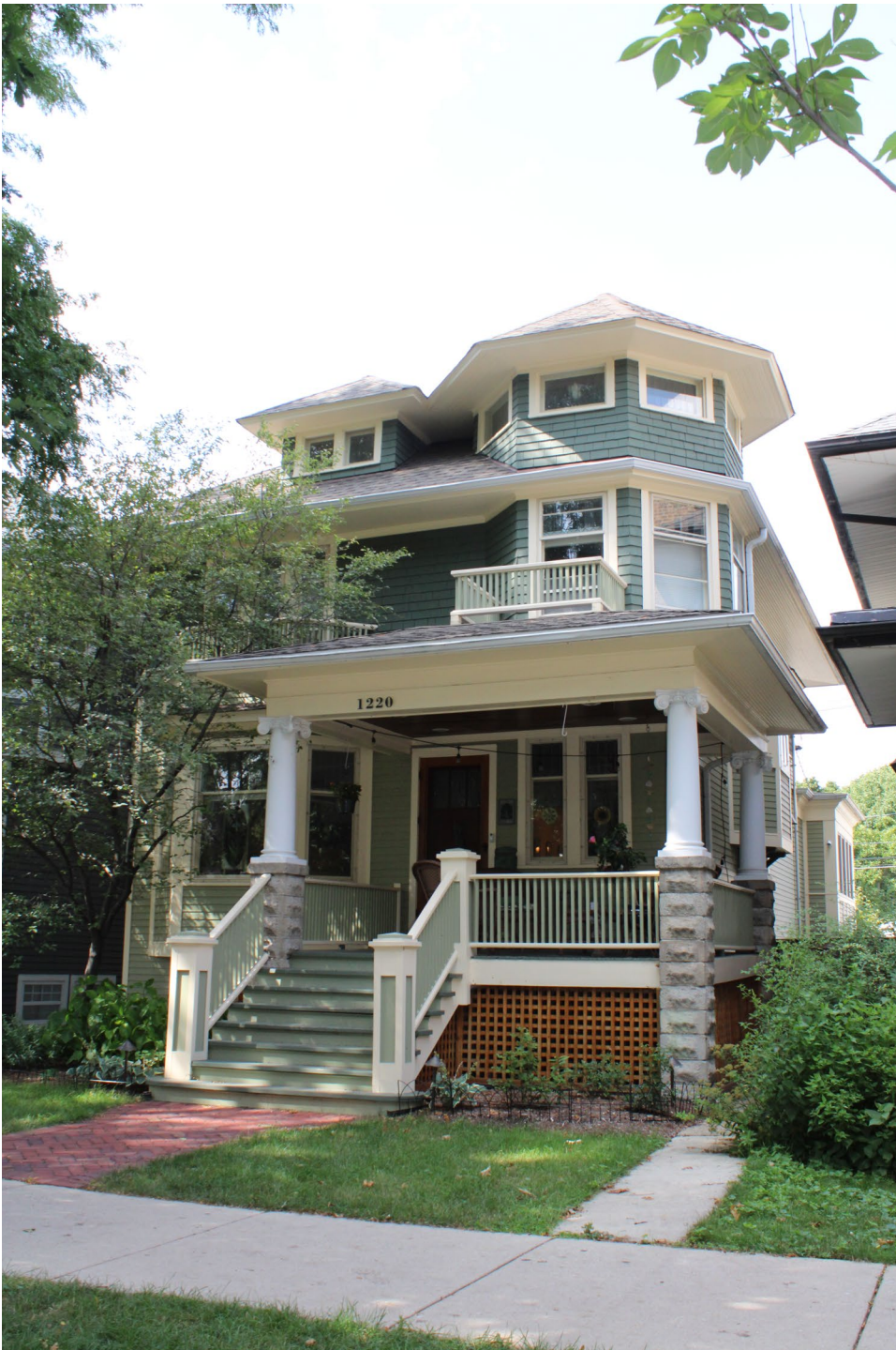
IMAGE 4: 1220 W. Glenlake Avenue: An example of a hip-roof, Queen Anne style house with partial-width porch, hip roof, and polygonal corner turret topped with a conical roof.
